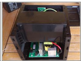
Remove left/right clips. And remove the bottom pannel
