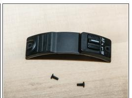
Unscrew the two screws holding the focus switch plate. The plate should just fall off.
