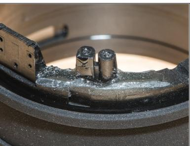
Try not to get glue down the outer side of the support stud. Excess glue will interfere with reassembly later. If glue does get in the wrong place, carefully grind it down with a dremel tool once it hardens.
