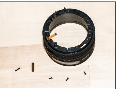
Remove the three screws around the outer ring. Lift off the zoom ring assembly. Don't snag the ribbon cables.
