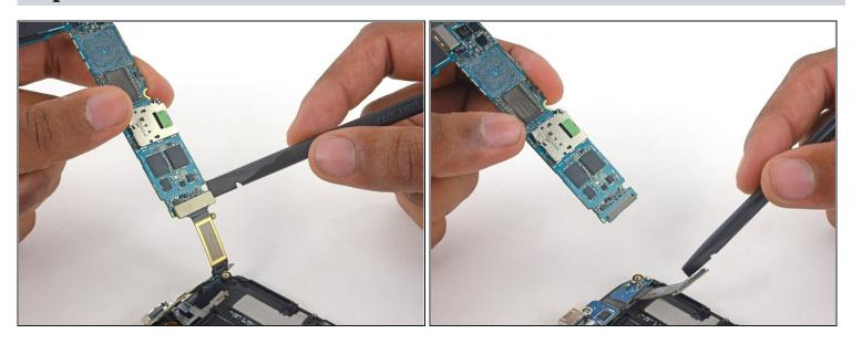
• Use the flat end of a spudger to disconnect the daughterboard ribbon cable connector from its socket on the underside of the motherboard.
