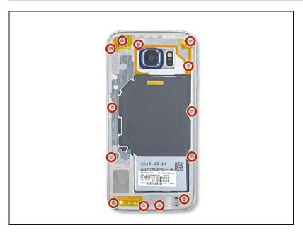
• Remove the thirteen 3.5mm Phillips #00 screws securing the midframe to the phone.
