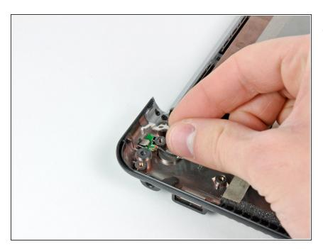
Remove the steel sleep switch bracket from the lower case.
