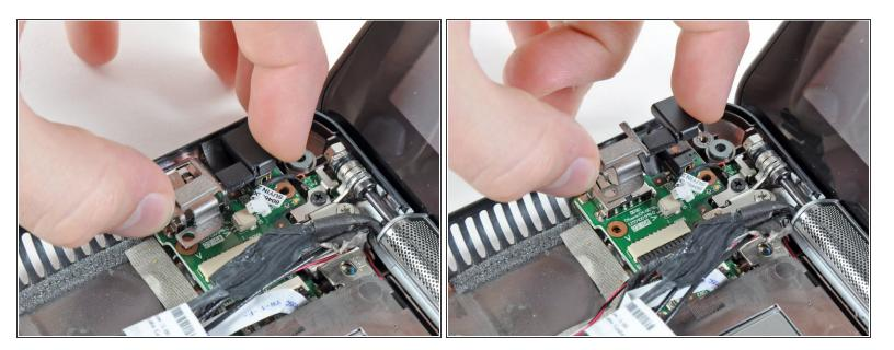
Lift the DC jack bracket up off the USB and power board.
