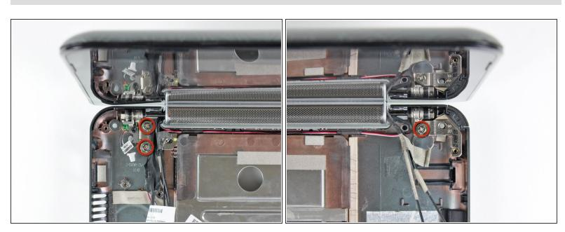
• Remove the three 5 mm Phillips screws securing the display assembly to the lower case.
