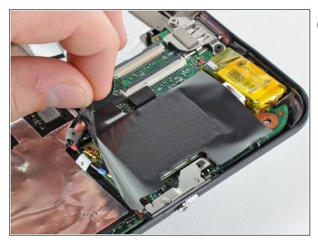
if present, carefully peel the piece of tape covering the WWAN board.
