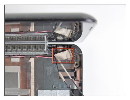
If present, peel back the piece of silver cloth tape covering the right display hinge.
