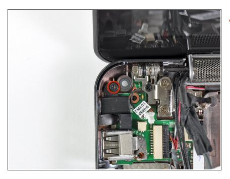
Remove the single 3 mm Phillips screw that secures the USB and power board as well as the DC jack bracket to the lower case.
