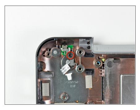
Remove the single black Phillips screw securing the sleep switch to the lower case.
