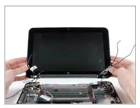
Remove the display assembly, minding any cables that may get caught or are still taped down to the lower case.
