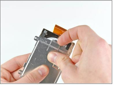
Lift up the center retaining tab on the hard drive enclosure and simultaneously push the hard drive out through the open end of the enclosure.
