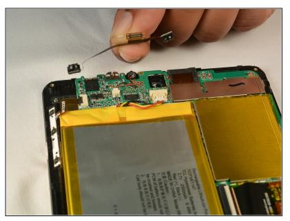
• Lift the camera assembly away from the device to remove it.
