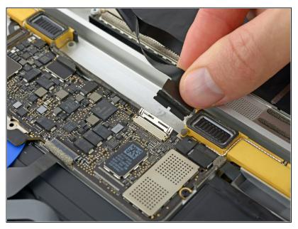
Disconnect the display cable by gently pulling it straight out of its connector.
