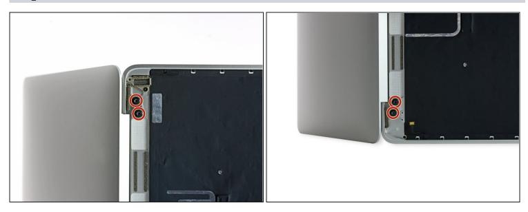
Remove the four 4.8 mm T8 Torx screws securing the display hinges.
