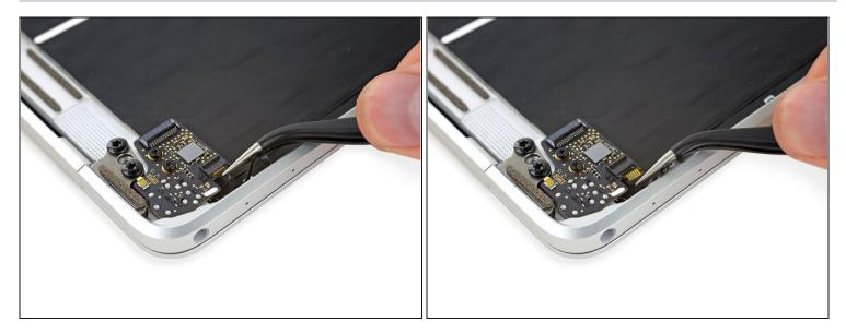
• Use <u>tweezers</u> to pull the microphone assembly ribbon cable free of its connector.
