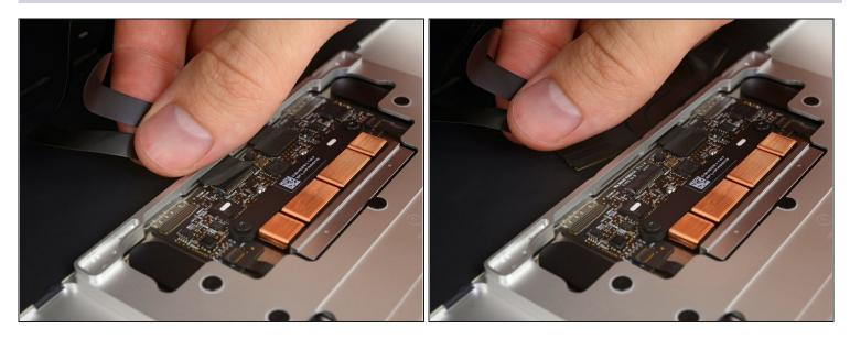
• Disconnect the trackpad ribbon cable from the trackpad by pulling it gently through its slot in the frame.
