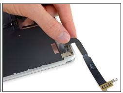
• Unfold the USB-C port ribbon cable until it lays flat, allowing access to the bracket beneath.
