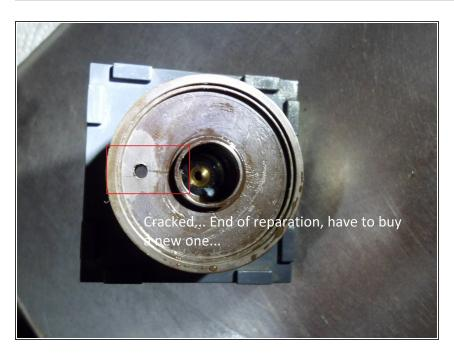
...and then I found a crack in my piston. That can not be repaired. So I had to buy a new piston.
