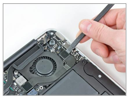
Use the flat end of a spudger to pry the I/O board cable connector upward out of its socket on the I/O board.
