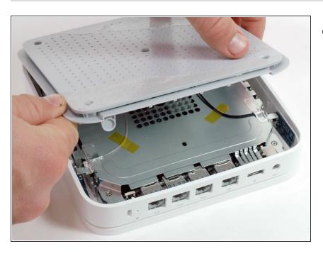
Lift the perforated plastic cover out.
