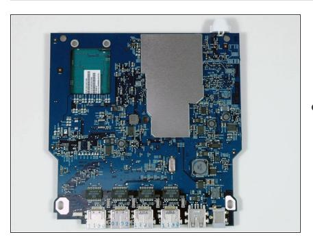
This is the bottom of the logic board. Not much to see here--something large covered by another heat sink. At the top right is a plastic cover over the LED. Four ethernet ports, one USB port, a power jack, and a reset button. The Apple part number on the airport card is 603-9396-A.
