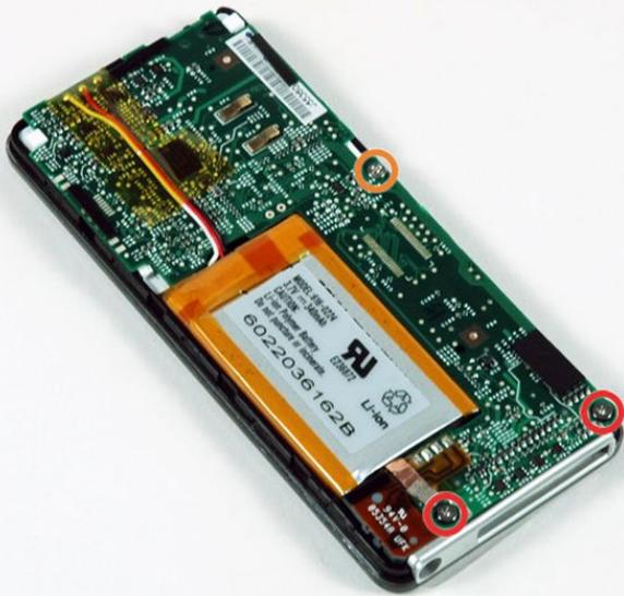
**i** Remove any kapton tape over the screws, if necessary.
