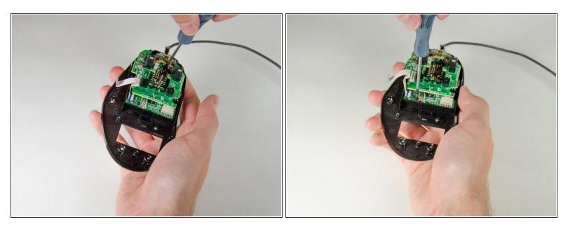
• Remove two screws securing the bottom circuit board to the bottom plate of the mouse.
