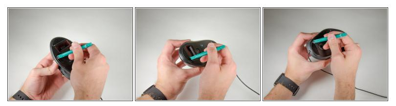
• Pry off the three feet to reveal screws.
