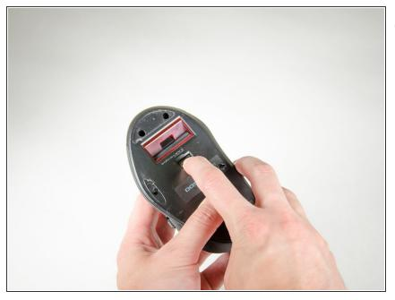
(i) Now, or at any time, you may wish to remove the weighted cartridge inside of the mouse. It is best if you do it at or before this step, but it is not necessary.
