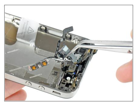
Grab the headphone jack with a pair of tweezers and remove the assembly from the iPhone, being careful not to rip the thin ribbon cables.
