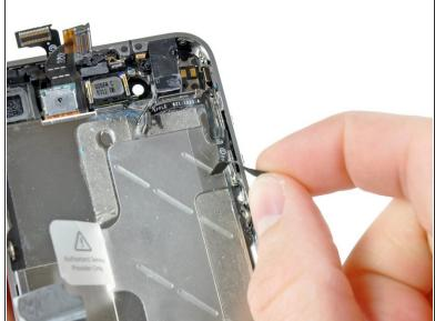
Use the edge of a plastic opening tool to peel the small strip of black tape off the back of the volume button bracket.
