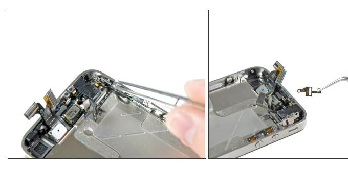
Use a pair of tweezers to carefully pull the silent switch and its bracket from the side of the outer case.
