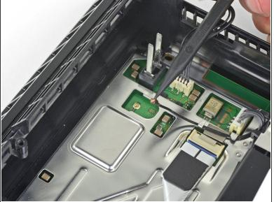
Use the tip of a spudger to disconnect the antenna cable from the motherboard.
