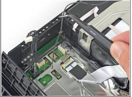
• Use a pair of tweezers or your fingers to thread the antenna cable out from underneath the optical drive cable.
