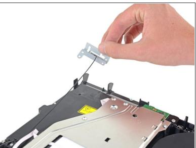
Remove the Wi-Fi antenna.
