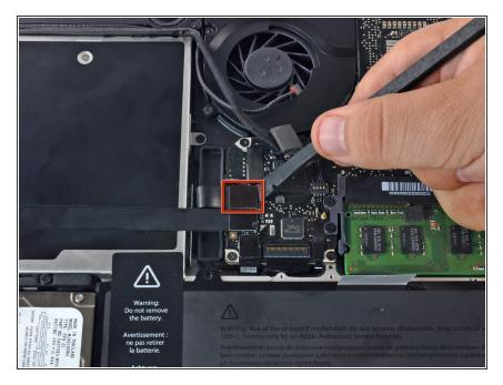
Use the flat end of a spudger to pry the optical drive connector straight up off the logic board.
