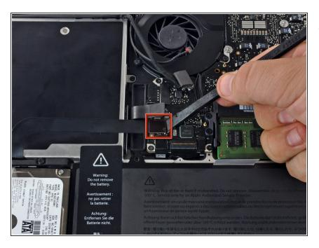
Use the flat end of a spudger to pry the hard drive connector straight up off the logic board.
