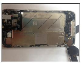
• Use the ifixit opening tool to remove the screws that hold the logic board in place and lift it with sprudgers in order to completely remove it from the Iphone (This will require some force when lifting the logic board).
