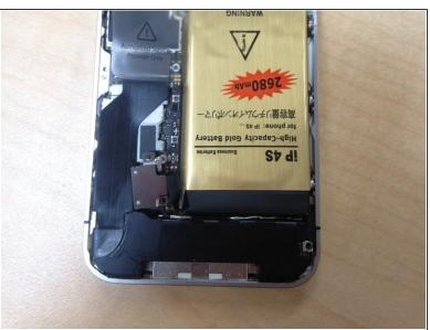
The iPhone will open up and you will see a metal panel by the camera on the top left side of the phone as well as a smaller metal panel on the bottom left side of the phone. These are required to be removed before taking out the battery. A Phillips #000 screwdriver will work best for removing them.
