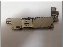
There will be the EMI Shields on the logic board (metal on top of the main processing chips) Which a spudger or the opening tool could be used for removal by lifting the small multiple metal tabs on the sides.(This will require <u>a lot</u> of force to lift off the logic board) (May cause a cut if not done without caution)
