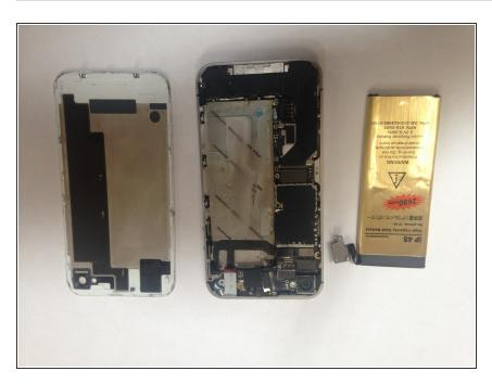
You'll automatically see the battery when taking of the back glass(will show a recycle sign and Li-ion written across). There is a plastic tab for you to use to help carefully lift the battery out of the phone (The battery has a connected wire to it, but it can be easily disassembled).
