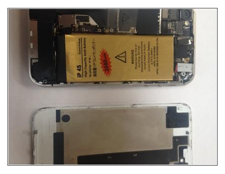
Make sure to <u>push up</u> on the back glass when taking it off (<u>be careful</u> if the back glass is cracked, loose glass could come off and potentially cut your hand if not done right)
