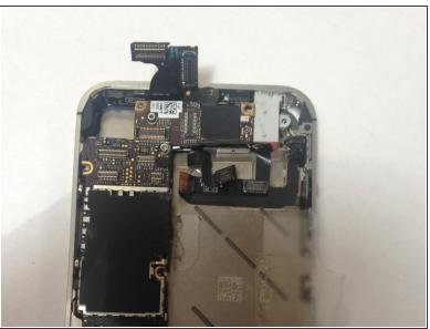
This is where you'll need your spudger, this will help you lift and disconnect your camera as well as other connectors which you can remove with tweezers (delicate part). With your spudger, you will go <u>under</u> the connector in order to lift and remove the camera from the logic board.
