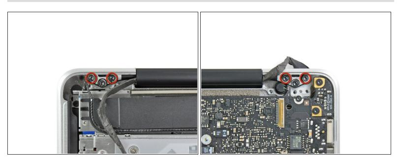
Remove the two outer 6.5 mm T8 Torx screws securing each of the two display brackets to the upper case (4 screws total).
