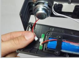
Remove all cable connectors from the speaker motherboard.
