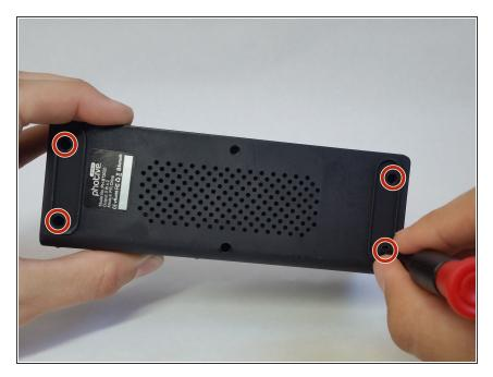
Remove four 9mm Phillips #0 head screws from the bottom of the speaker.
