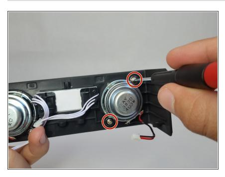
Remove two 7mm Phillips #0 head screws from the front panel.
