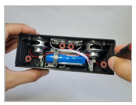
Remove four 9mm Phillips #0 head screws from the inside of the speaker case.
