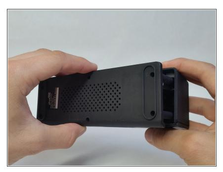
• Separate the base of the speaker from the upper housing.
