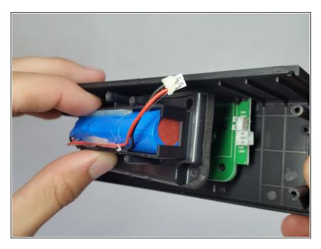
• Lift the battery pack from the board.
