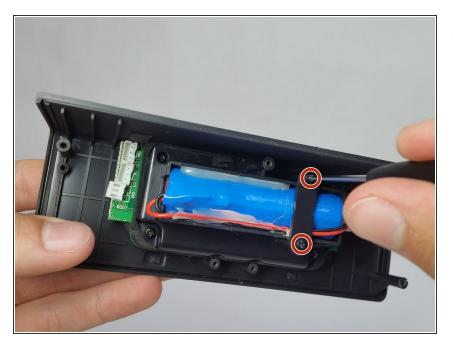
Remove two 9mm Phillips head #0 screws from the battery holder.
