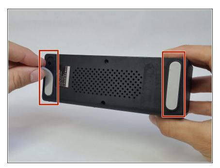
• Peel back the rubber feet from either side of the base.
