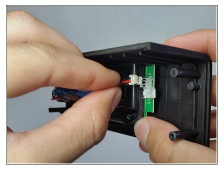
• Disconnect the battery cable from the motherboard.
