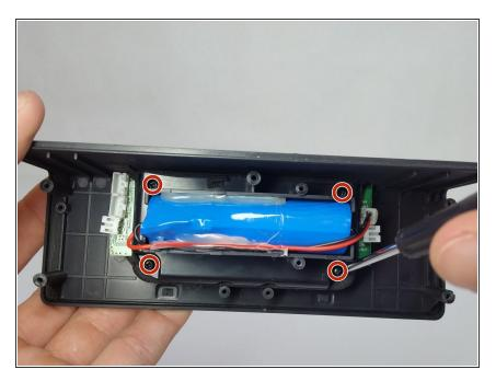
Remove four 9mm Phillips #0 head screws holding the battery pack in place.
