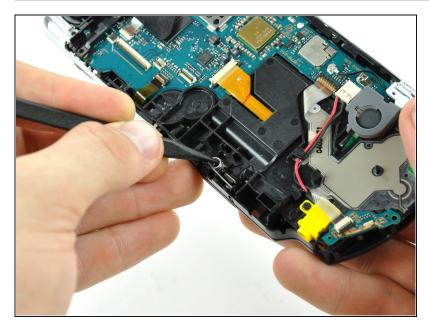
Using the pointed end of a spudger, pull the UMD door spring to the left, and remove it from the PSP.
