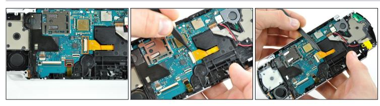
• Use your fingernail or the edge of a spudger to flip up the retaining flap on the UMD drive ribbon socket.
