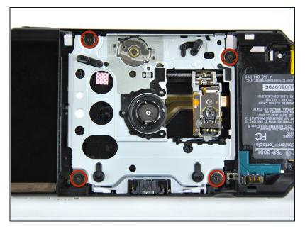
Remove the four Phillips screws securing the UMD drive to the PSP 300xc.
