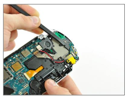
Using the flat edge of a spudger, pry the power board away from the PSP 300xc.
