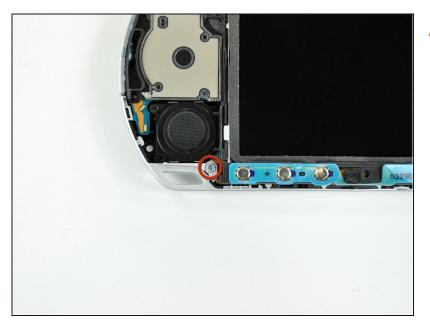
Remove a single Phillips screw securing the home bar to the PSP 300xc.
