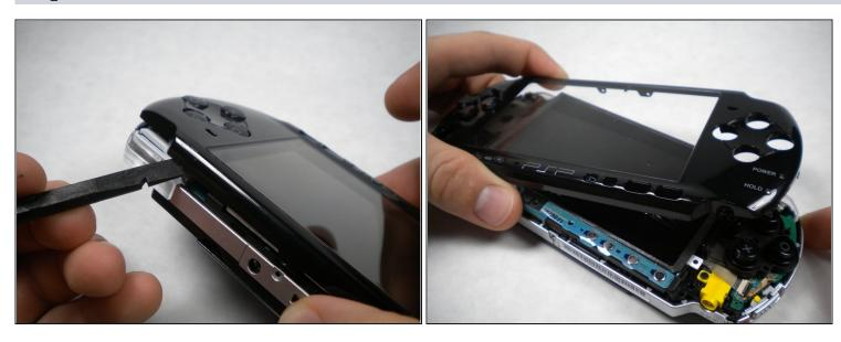
• Insert a spudger between the front case and PSP, and slide the spudger along the perimeter of the front case to remove it.
