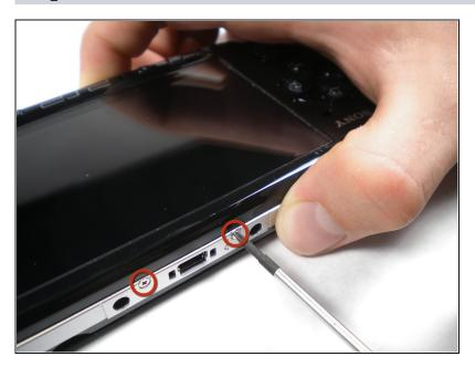
• Remove two Phillips screws from the top of the PSP.
