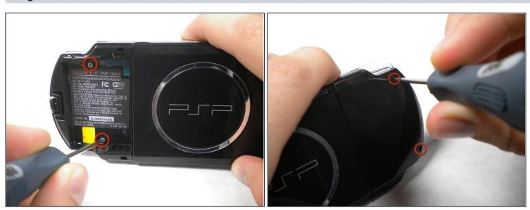
Remove four Phillips screws from the back of the PSP.
