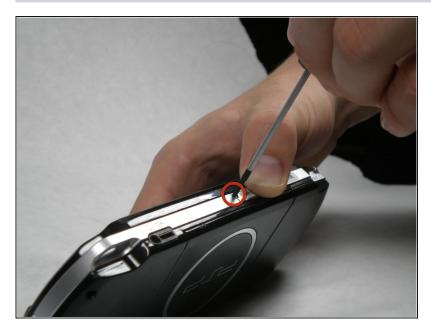
Remove a single screw from the bottom edge of the PSP.
