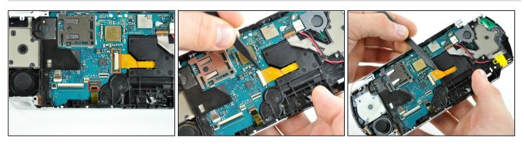
• Use your fingernail or the edge of a spudger to flip up the retaining flap on the UMD drive ribbon socket.
