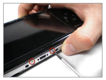
• Remove two Phillips screws from the top of the PSP.
