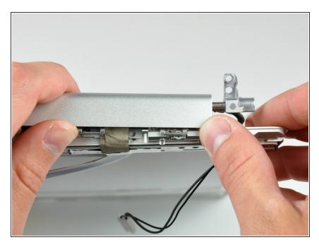
Repeat this process for the other side of the clutch cover. Once the clutch cover is completely free from the clutch hinges, lift it off the front display bezel.
