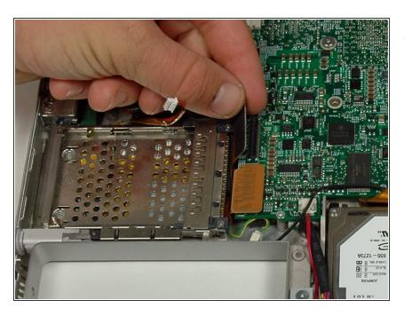
Disconnect the PC card cable from the logic board.
