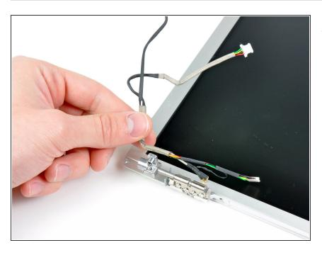
De-route the inverter/antenna cables from the left clutch hinge and lift them out of your display.
