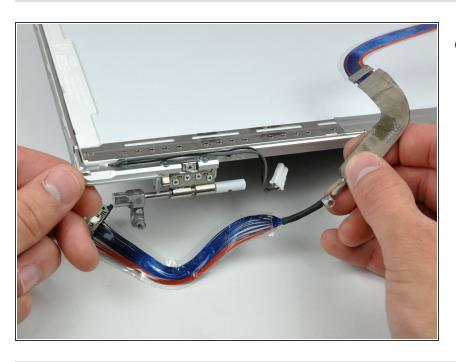
De-route the display data cable from the right clutch hinge and lift it out of the display.
