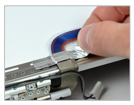
Remove the piece of foil tape securing the display data cable to the LCD frame.
