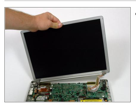
Lift the display assembly off the lower case.
