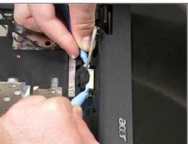
Detach the white rectangle located on the motherboard at the end of the wire connected to the LCD screen.
