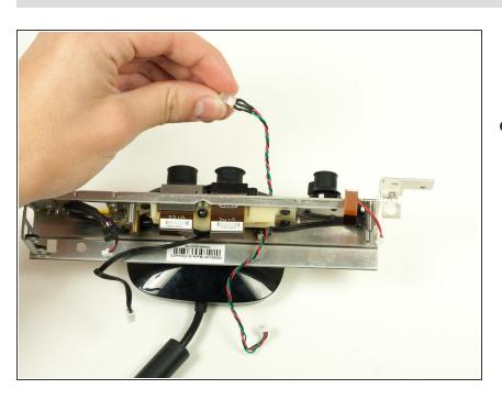
Gently pull the LED out of the front of the metal casing. It should slide out easily.
