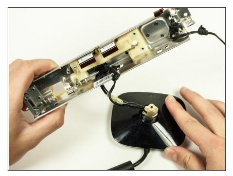
Carefully remove the top body portion of the Kinect from the stand by guiding the cable through the hole on the underside of the body, then lifting the body off of the plastic stand.
