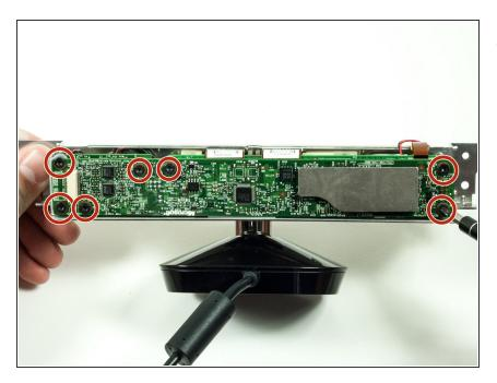
Unscrew the seven 6.5mm T10 Torx screws.
