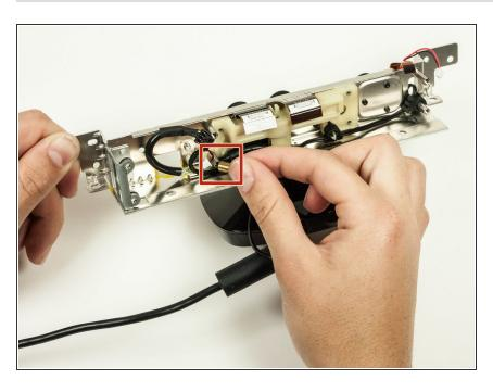
Remove the gold metal cylindrical piece from the metal body on the left side of the Kinect.
