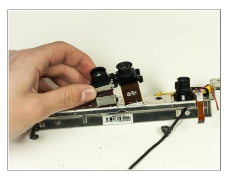
Remove the two cameras on the left (which are connected) by pulling their ribbon cables through their respective slots.
