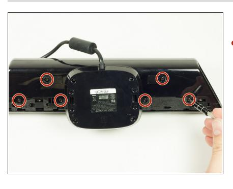
Unscrew the six 12mm T10 Torx screws.
