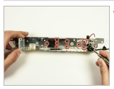
Unscrew the nine 7mm T6 Torx screws from the metal body. These hold the cameras in place.
