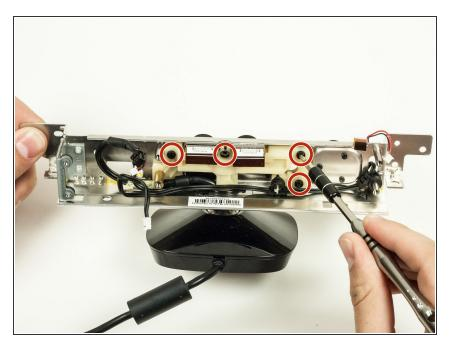
Unscrew the four 7mm T10 Torx screws from the plastic body.
