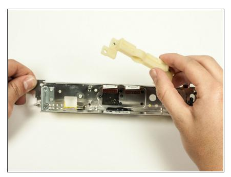
Remove the plastic body from the metal body by sliding it off of the metal cylinders.
