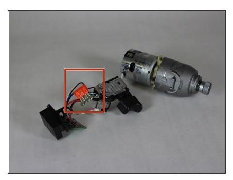
Identify the translucent orange fuse cartridge connected by a thick red wire and a thick white wire.
