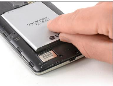
Use a fingernail or a prying tool at the marked notch to lever the battery out of its recess.
