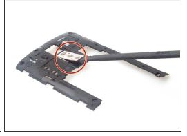
Using the spudger, release power & volume button flex from adhesive carefully.
