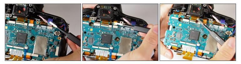
• Use tweezers to disconnect the blue, gold, and brown ribbon connectors near the top of the camera.
