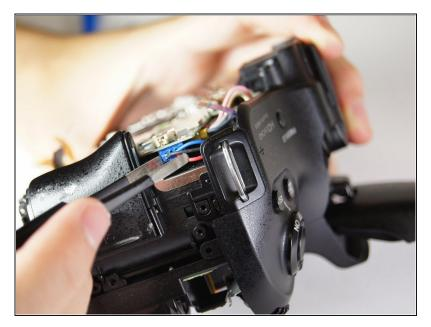
• Use tweezers to unplug the blue adapter located at the top right of the circuit board.
