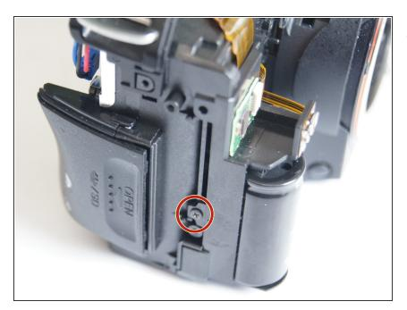
Remove the 5.0 mm Phillips #00 screw on the left side of the camera next to the flash capacitor.
