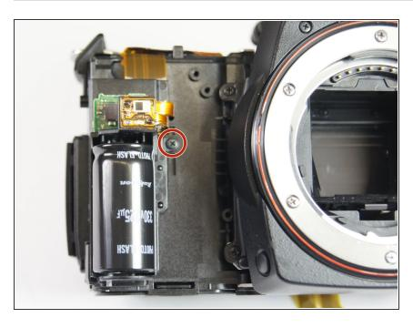
Remove the 5.0 mm Phillips #00 screw on the right side of the flash capacitor.
