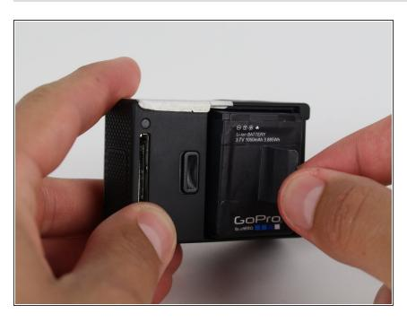
Pull the battery out using the tab.
