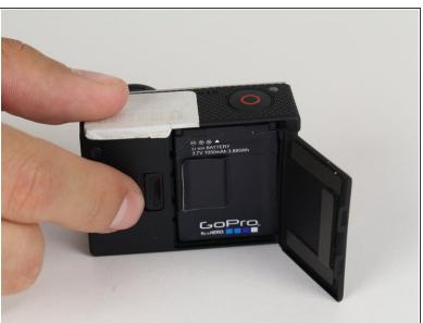
Pull back on the tab on the back of GoPro to open the battery cover.
