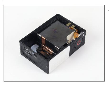
In order to replace the buttons. The entire housing has to be replaced. To reassemble your device, follow these instructions in reverse order.
