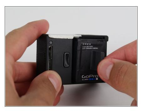
Pull the battery out using the tab.
