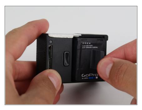
Pull the battery out using the tab.
