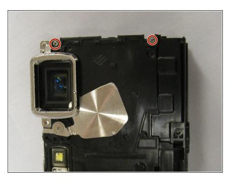
Using a Phillips 00 screwdriver, unscrew the 9mm screws on the top of the camera to the right of the flash.
