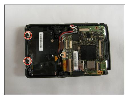
Unscrew screws on place holder plates
