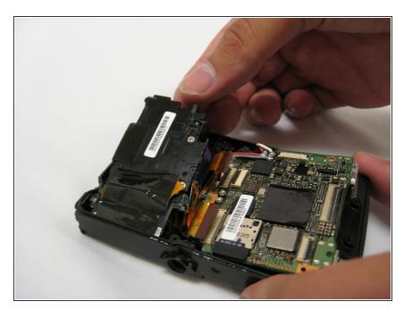
Gently lift Lens compartment out of device.
