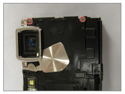
Using a Phillips 00 screwdriver, unscrew the 9mm screws on the top of the camera to the right of the flash.
