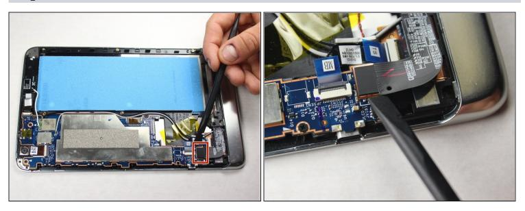
Locate the LCD cable connector and gently pry it directly up with a spudger.
