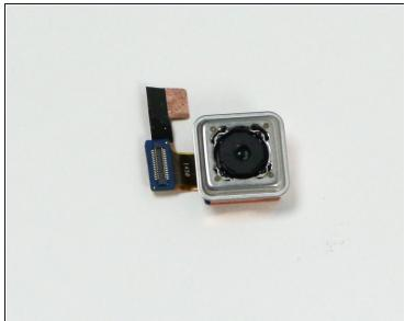
• Flip the daughterboard over and use the tweezers to remove the back camera from the board by applying upward force to the ribbon connection.
