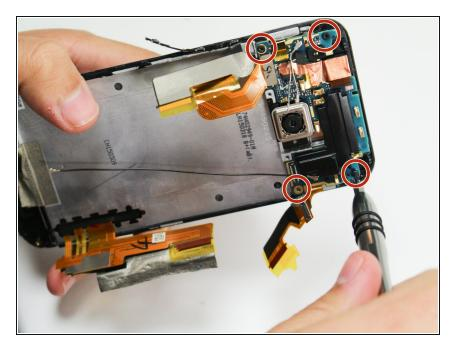
Remove the four 3 mm T5 Torx screws that secure the daughterboard.
