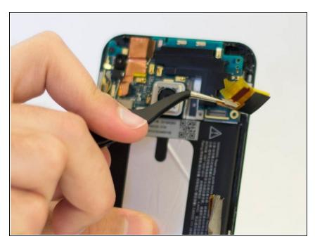
• Using the tweezers, disconnect the ribbon cable.
