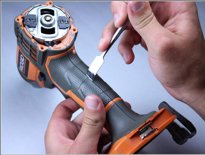
**⚠** Place the driver flat on a table before completely separating the two halves of the housing so components of the drill don't fall out during opening.
