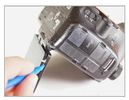
Use the plastic opening tool to gently pry the screen open around the entire screen.
