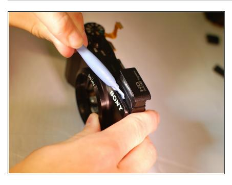
From the top of the camera, Use a plastic opening tool between the flash and the case to remove the flash.
