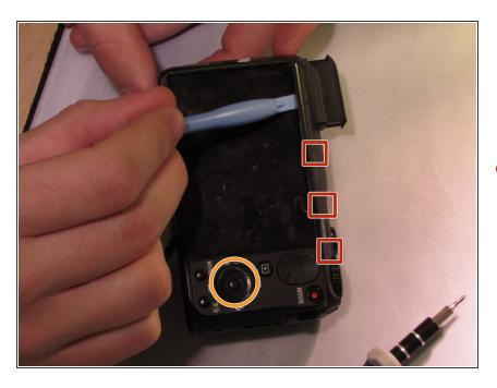
Use the plastic opening tool with a prying motion, going between the case and the LCD, from the middle
