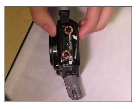
After removing the panel, remove the two black M1.4 X 3.5 Phillips head screws.
