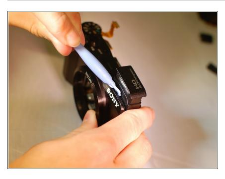
From the top of the camera, Use a plastic opening tool between the flash and the case to remove the flash.
