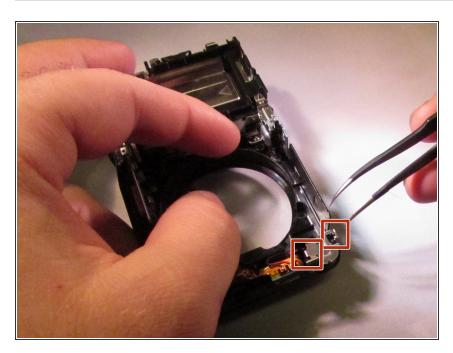
Use tweezers to remove the speaker retaining clip. The retaining hooks locations are indicated, but not exact.
