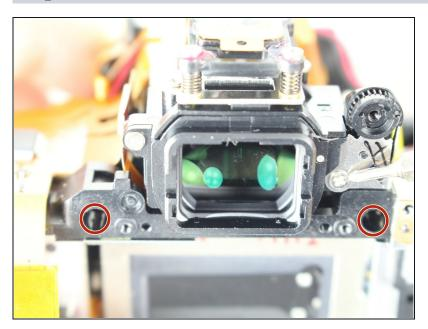
Remove two screws from just below and to the sides of the viewfinder.
