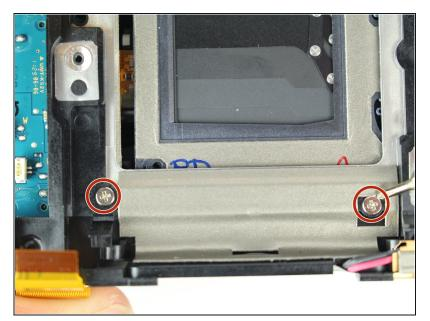
• Remove two 6 mm J000 screws from the left of the shutter.
