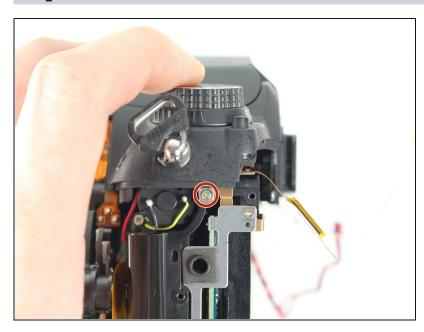
Remove one 4 mm J000 screw securing the top case (under right strap hook).
