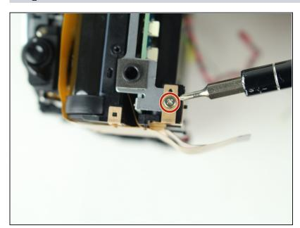
Remove one 3 mm J000 screw from the bottom left side of the camera.
