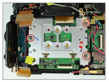
Remove three 6 mm J000 screws securing the image sensor.
