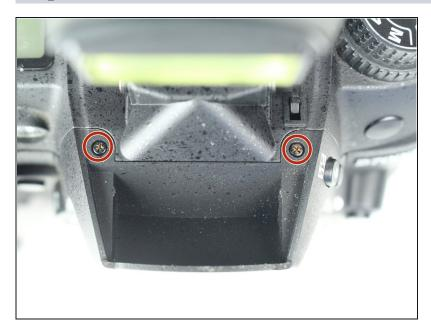
• Remove two 5 mm J000 screws from under the flash.
