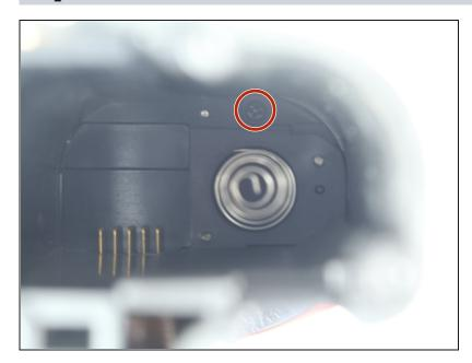
• Remove one 8.5 mm J000 screw from the battery compartment.
