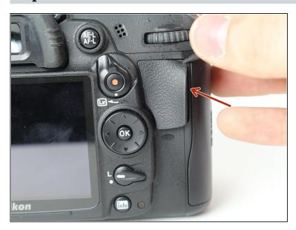
• Peel the rear rubber piece off with <u>tweezers</u>.
