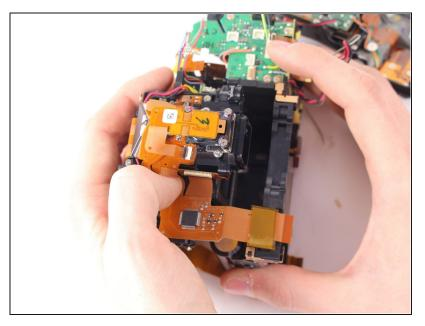
• Separate the shutter assembly from the camera body.
