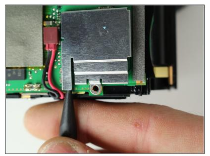
• Gently lift the right motherboard shield off with the tip of a spudger.
