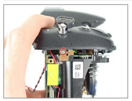
Remove one 4 mm J000 screw securing the top case (under left strap hook).
