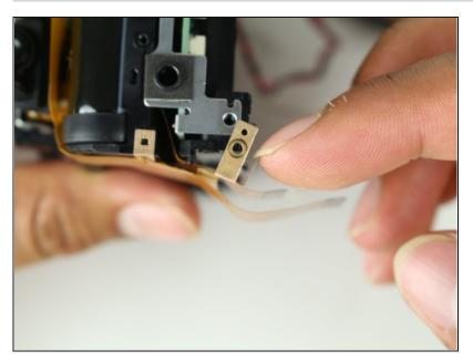
Carefully peel back ribbon cable on the bottom left of camera.
