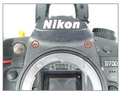
Remove two 3 mm J000 screws securing the front cover.
