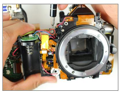
Remove one 5 mm J000 screw from the top right of the camera.
