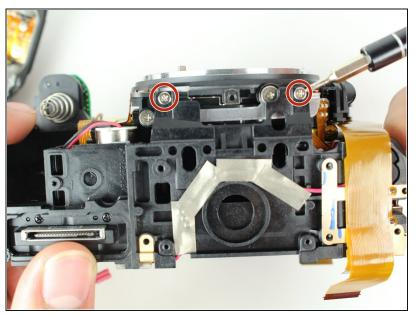
• Remove two 6.5 mm J000 screws from beneath the lens mount.
