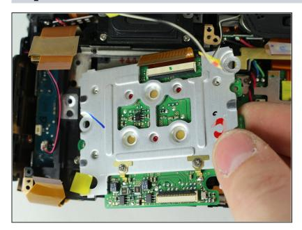
Carefully lift the image sensor plate out of the camera.
