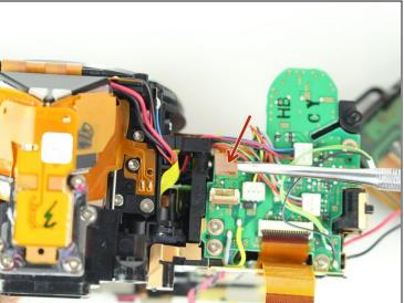
• Remove the left front ribbon cable from top right of circuit board.
