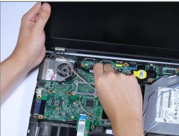
Unplug the two black cables that connect the screen to the motherboard.
