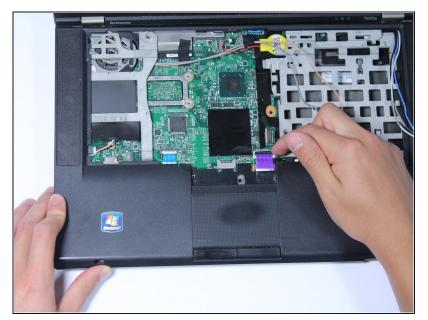
Lift up the black retaining flap holding the purple ribbon cable in place, and carefully slide out the ribbon.
