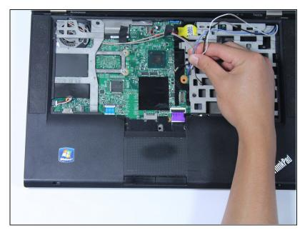
Flip the laptop back over and pull all the wires from the previous step through to the top side.
