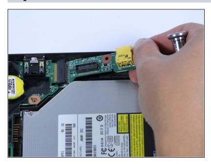
• Lift the power jack and slide to the right to remove.
