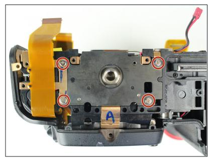
• Remove four 6 mm J000 screws securing the tripod plate.
