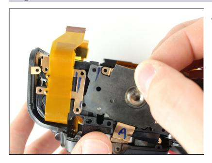
Carefully lift the tripod plate from the backside of the camera and slide out the grounding clip from under the lens mount.
