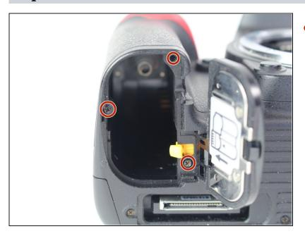
Remove three 6 mm J000 screws from under the battery cover.
