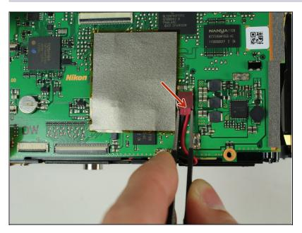
• Carefully disconnect the red connector with tweezers.
