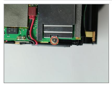
Remove one 3.5 mm J000 screw securing the right motherboard shield.
