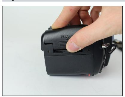
Open the SD card cover by pushing slightly down with your thumb and sliding up.
