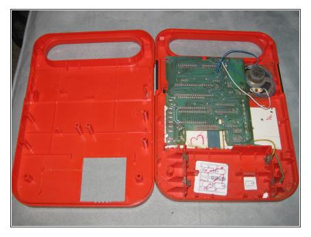
Separate the two halves of the case to expose the inner PCB, speaker and battery holder.
