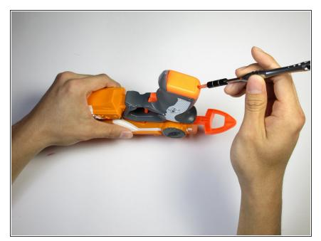
Use a #1 Phillips screwdriver to remove the 10 -mm screw that secures the battery plate, then remove the battery cover using your hands.
