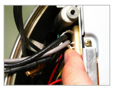
Release the Airport and Bluetooth cables from the white plastic clip, mounted to the upper left edge of
