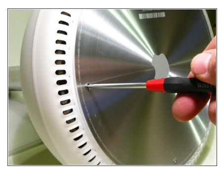
Loosen the (4) Phillips screws securing the User Access Plate to the iMac's Bottom Housing. the screws are captive and not removable.
