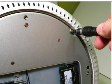
Remove the 4 Torx screws securing the Bottom Housing with a T15 Torxdriver.
