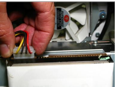
Disconnect the Hard Drive's Data and Power Cables, Pulling the Data Cable connector by its white plastic tab (not the cable itself), and the Power Cable by its outside edges. These connectors can be very tight. Don't get discouraged. Patiently wiggle them back and forth so that they release evenly to avoid bending any pin's.
