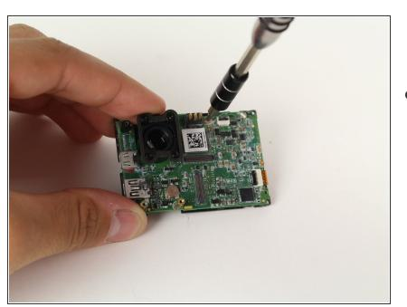
Using your trusty screwdriver, remove the single 3.2mm PH00 screw connecting the motherboard to the midframe.
