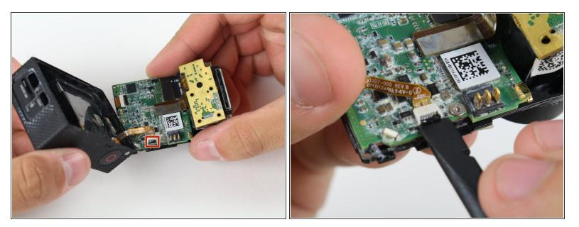
Remove the ribbon cable connecting the housing to the motherboard by flicking up the black clip with the spudger tool and gently pulling the cable out.
