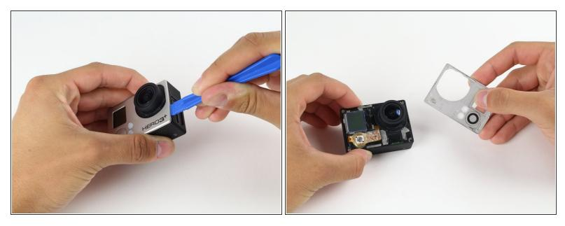
Using a plastic opening tool, pry the gray, front face plate until it can be removed from the housing.
