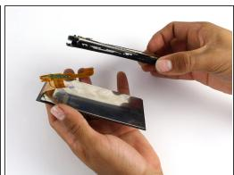
• Carefully guide the display assembly ribbon cable through the midframe for removal.
