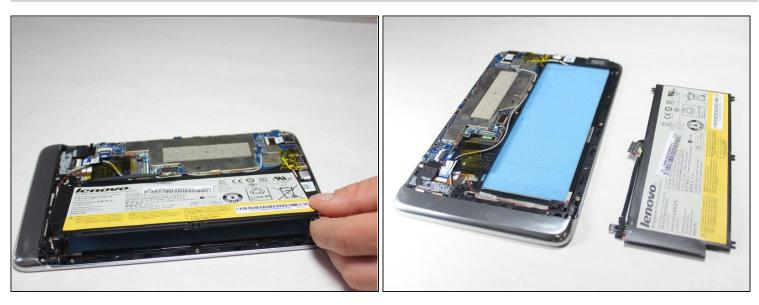
• Remove the battery by prying up with your fingers or a plastic opening tool.
