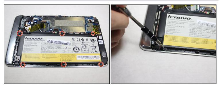
Unscrew the six 3mm screws surrounding the battery dock using a Phillips #0 screwdriver.
