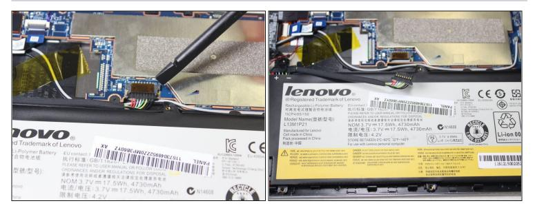
• Using a plastic spudger, slowly push each side of the battery connector (back and forward a couple of times) out of its socket on the motherboard.
